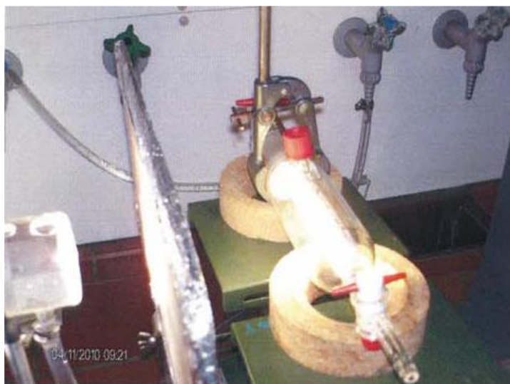
Fig.1: Photoreactor with water filter for the removal of infrared rays (centre).
